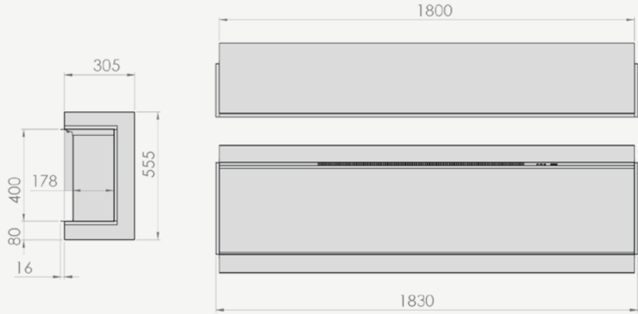
iRANGE i1800E - OVERALL UNIT DIMENSIONS (MM)
