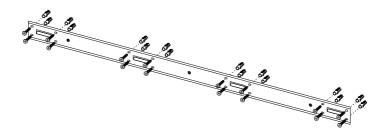
Attach the bottom mounting brackets to the appliance using four ST4x8 screws provided.
