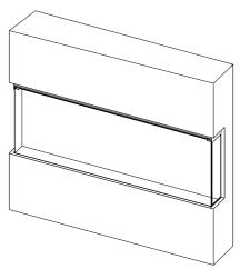
Remove two screws securing the glass retaining clip to remove the front glass for arranging the fuel bed. Use the suction cups provided to support the glass panel and carefully lift it away as shown below.
