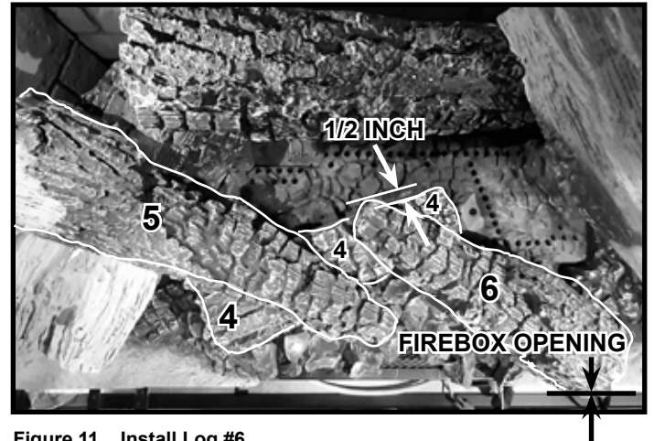
Figure 11 Install Log #6
