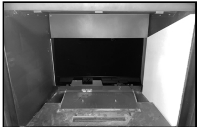
Figure 7 Rear Glass Panel and Side Insulation Board Installed
