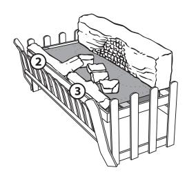
3. LOCATE LOG NO'S 2 & 3: Two front log NO'S. 2 & 3 are supplied to fit into the space between the metal frame and the ceramic base. These logs do not cover the front burner ports but are designed to deflect the front flame back into the fire.
