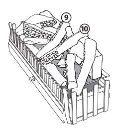
6. LOCATE LOG NO. 9. This log is placed on the rear log in the centre of the burner. Charred effect facing toward the left of the burner. The front rests on logs 2 & 3 on the join.
