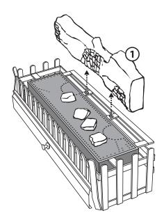
2. LOCATE LOG NO. I: This is the largest log that is positioned at the rear of the grate. Two locating pins are positioned at the rear of the burner. The large log has two holes on the underside to position in place.
