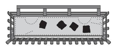
I. LOCATE 4 CERAMIC COALS: Four ceramic coals are supplied with the burner base. These coals must be laid in the position indicated on the drawing with the taller coals on the ends and smaller coals in-between.
