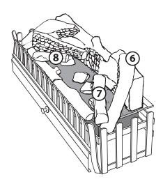
5. LOCATE LOG NO. 6. Place this log on the right hand side of the burner on the rear log in front of the pilot. Charred end facing inwards. The left hand side of the log is positioned between the metal uprights on the side of the grate.
